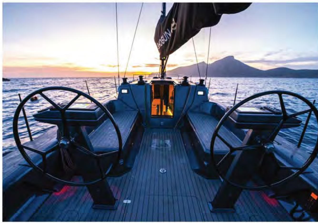
Above: the optional teak effect deck looks good but added 110kg of weight to the test boat
