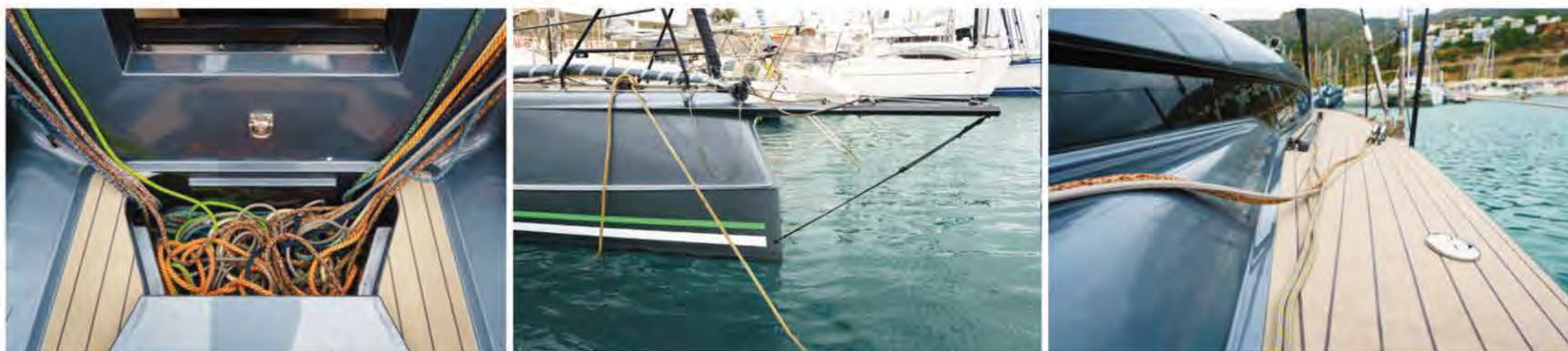
From left: large rope bins at the pit; angular lines melded to a long bowsprit for flying offwind sails; sheet leads include an outboard jib position
